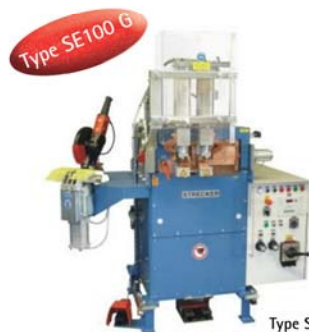
Type SE 100 G copper strands 5 - 1500 MCM aluminium strands 3 - 2000 MCM
